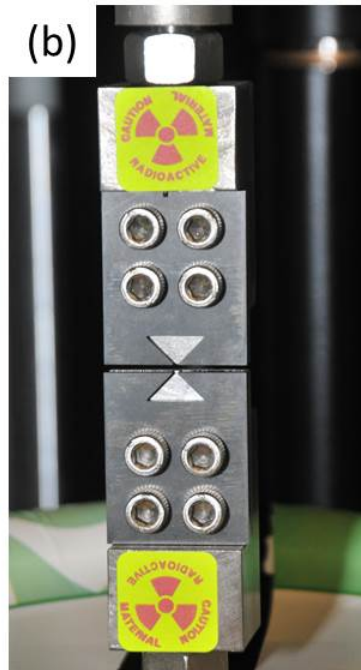
Figure 3.4: Photographs of low carbon steel mini tensile sample (a) and tensile test grips (b).
