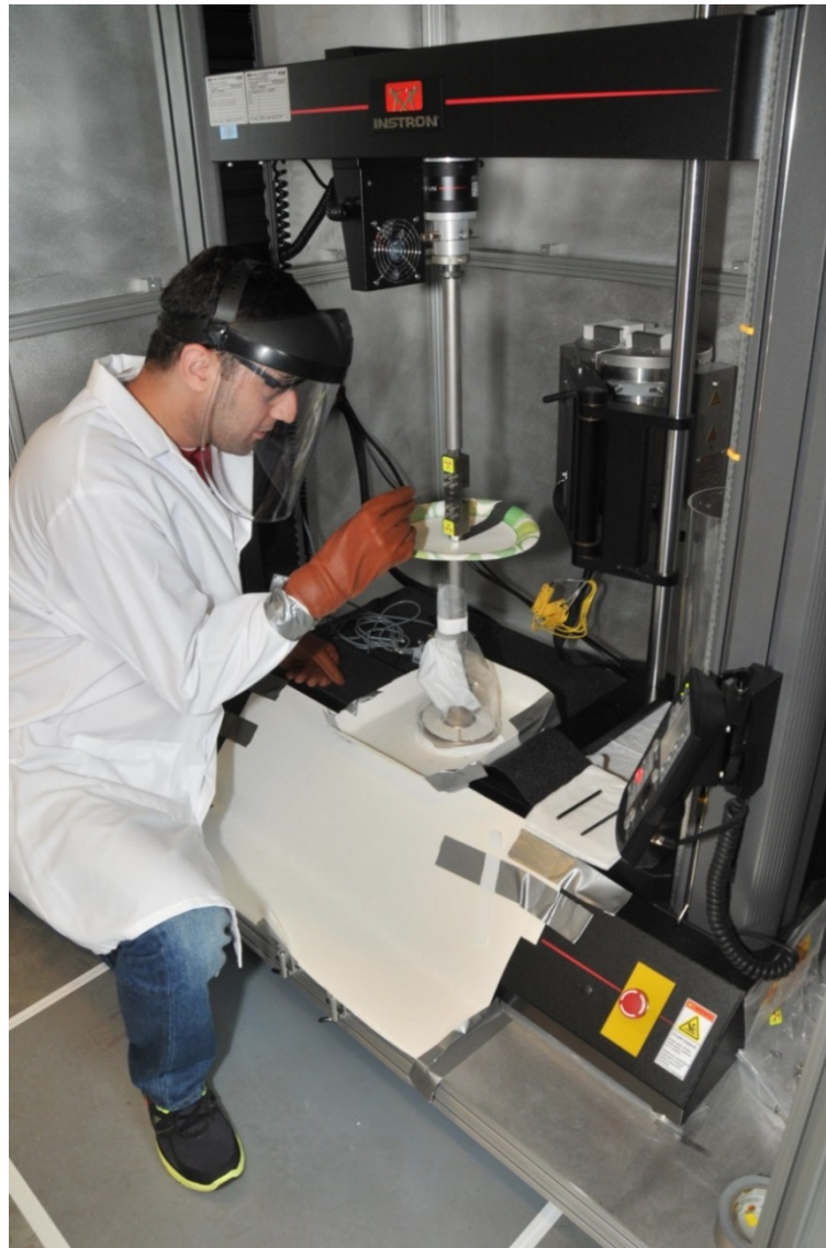
Figure 3.15: Tensile test for radioactive steel samples conducted at Center for Advanced Energy Studies (CAES) using Instron machine.
